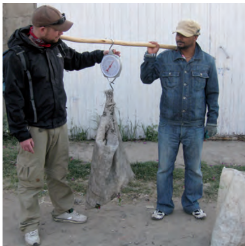
Lifting device – “Balance stick”
