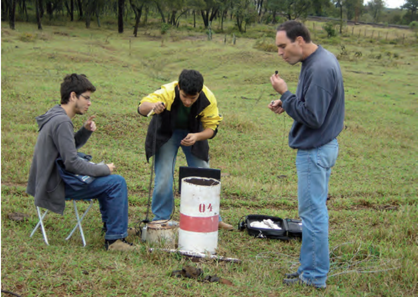
Groundwater level measurement in a monitoring well installed in the Guarani Aquifer outcrop zone
