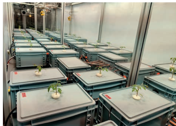
Test setup to investigate the optimum growth conditions depending on nutrient solution salt concentration levels at the Hohenheim University Phytotechnical Center
