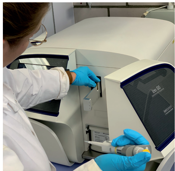
Virus-RNA from a wastewater sample is placed in the sequencer
