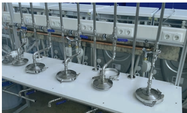
Washing tests are carried out to measure the extent of textile microplastic emissions. The picture shows the filter system and washing machines at the Niederrhein University of Applied Sciences.
