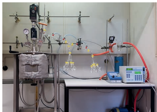
Laboratory reactor with attached condensation unit for the depolymerization of polystyrene
