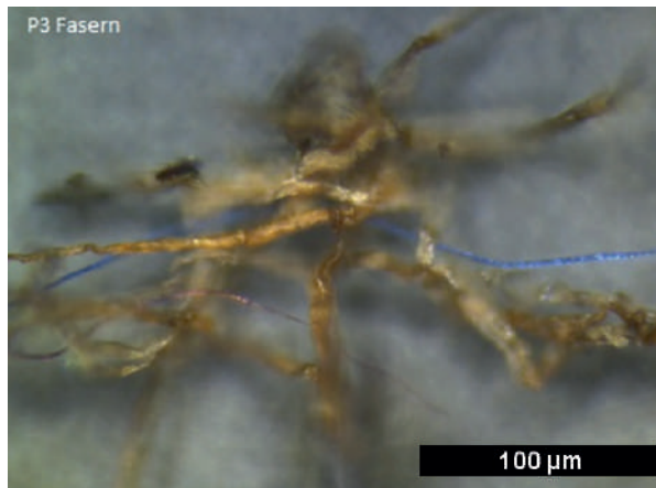
Microscopic image of plastic fibers whose biodegradability is being investigated in this joint research project.
