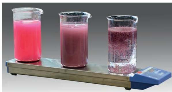
Flocculation of microplastics (left: suspended microplastics; middle: the flocculation process; right: microplastic flakes rising to the surface).
