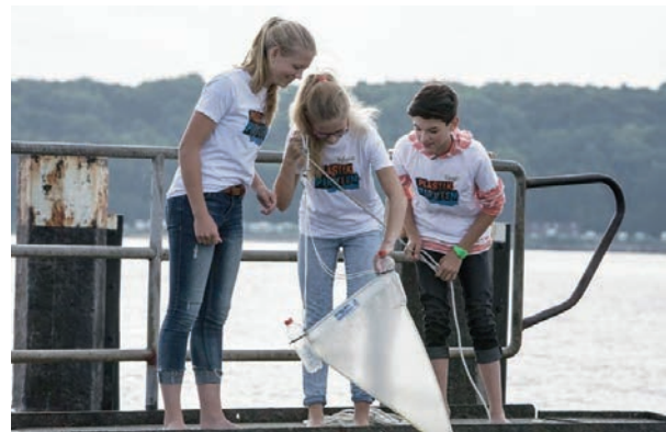
The plastic pirates take a water sample with a fine-meshed net in order to have it analyzed later for microplastics
