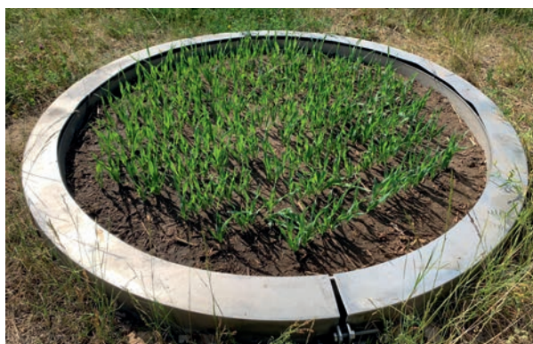
A soil core (lysimeter) planted with brewer's barley
