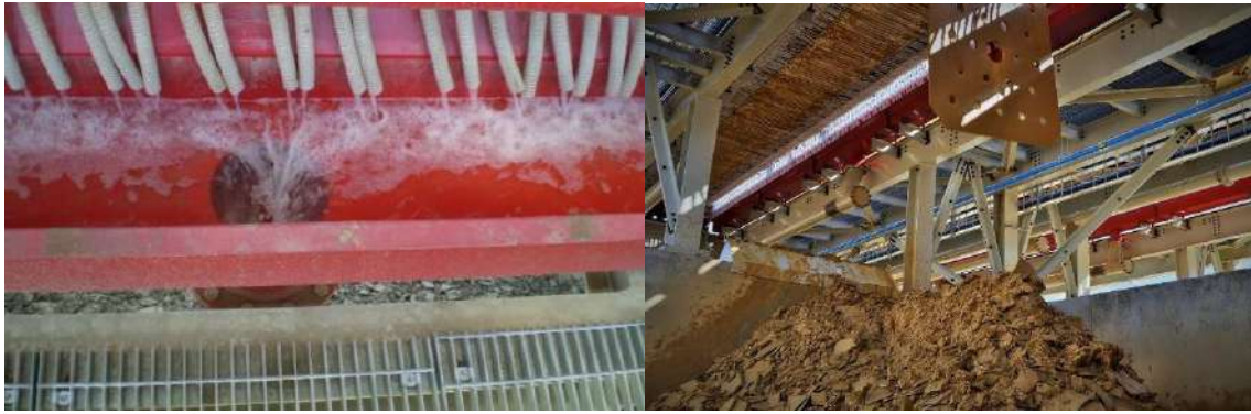
Figure 3: Dewatered cakes (tailings) discharge from a Filter Press into a pile (Zink, 2020)
