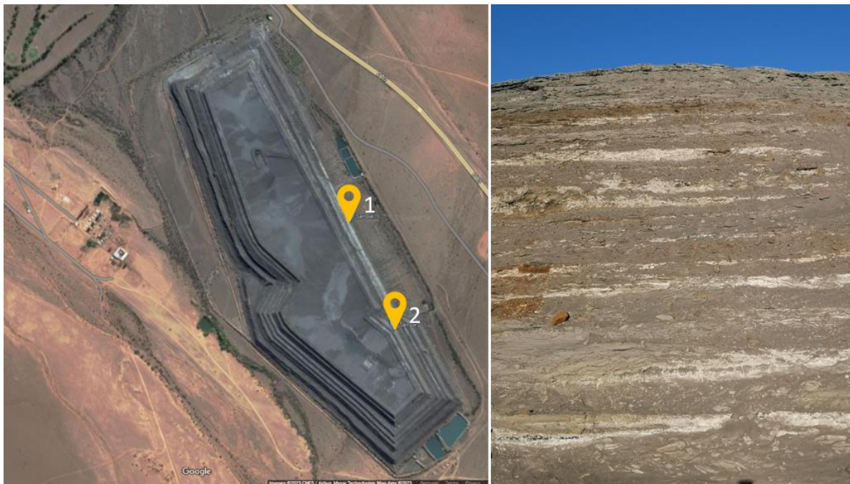
Figure 11 Locations of sampling points in the tailings dam (left). View of the stratified tailings (right).
