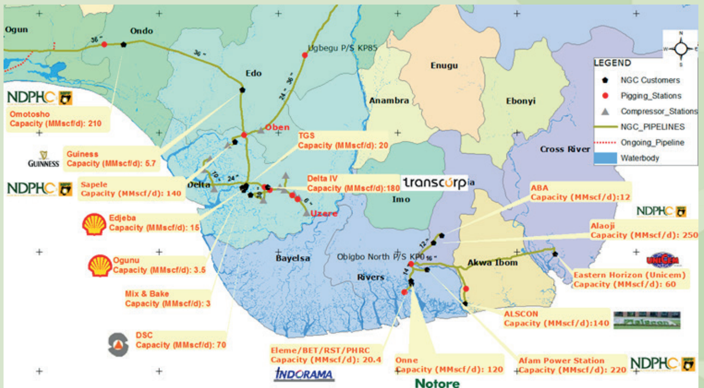
Figure 18: Map of Nigeria Existing Gas infrastructure including end users - Western and Eastern Gas Pipeline Networks [62]
