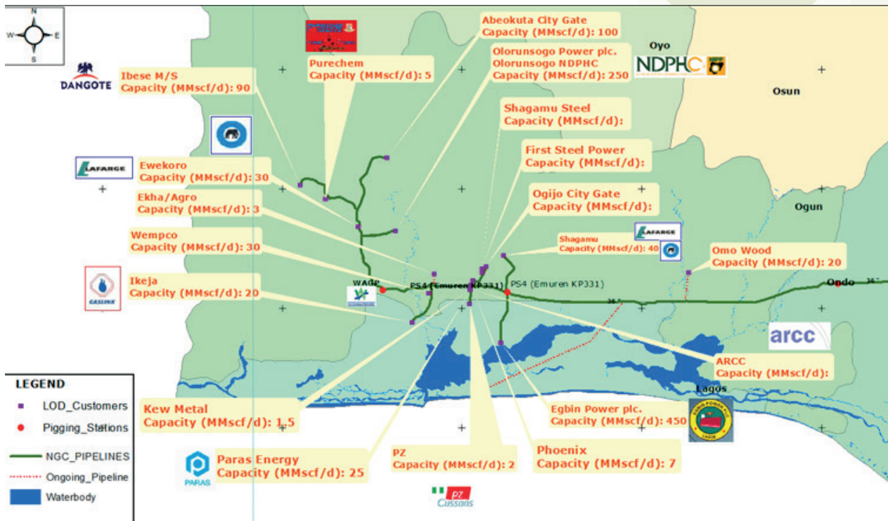
Figure 19: Map of Nigeria Existing Gas infrastructure including end users - Western Pipeline Network [62]
