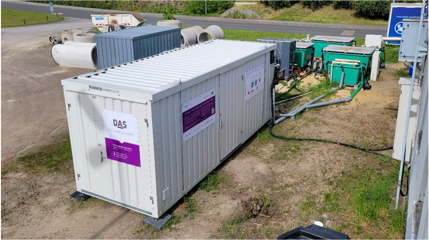
Pilot plant for the degradation of DMAC - in the foreground: MBBR container, in the background: vertical filter system (Source: Christian Koch, TU Dresden, Professur für Siedlungswasserwirtschaft)
