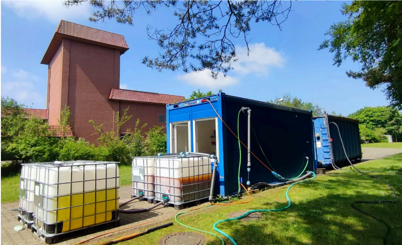
Pilot tests in the waterworks, with the test container in the center and two tanks containing concentrate from the membrane filtration of filter rinse water (Source: OOWV/DVGW research center TUHH)
