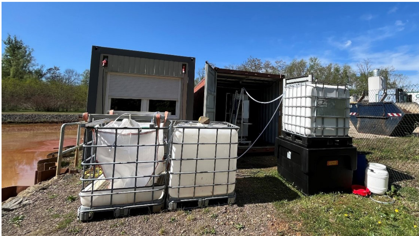
Installed SULFAMOS pilot plant at the field site of a water treatment plant. Right: Module for forward osmotic sulfate enrichment, left: module for sulfate separation by means of precipitation as gypsum (Source: G.E.O.S.)
