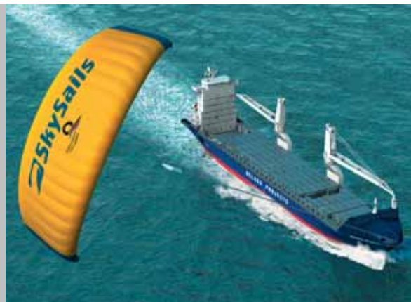
Left: SkySails towing kite system on the coastal vessel "MS Beaufort". Right: The illustration shows the system installed on a cargo ship.
